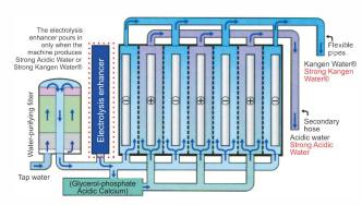
If you push the button for Strong Acidic Water, the secondary hose releases Strong Acidic Water and the flexible pipe releases Strong Kangen Water® at the same time.
